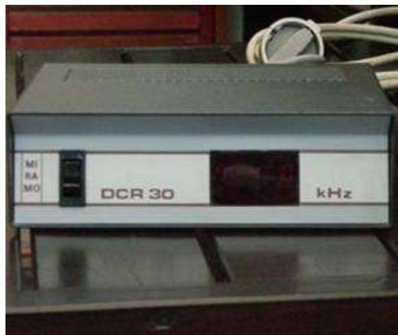
Accessory to show 0-999kHz. MHz value is read on the radio
